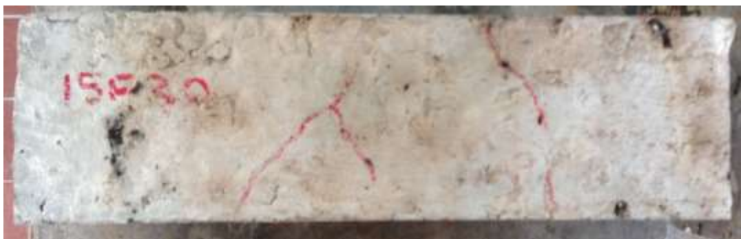
Figure 12: specimen after heating (300oC) in oven for two hours
