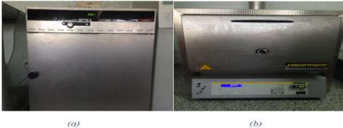
Figure 7: Heating Oven (a) For 50 and 70 o C, (b) For 300 o C
