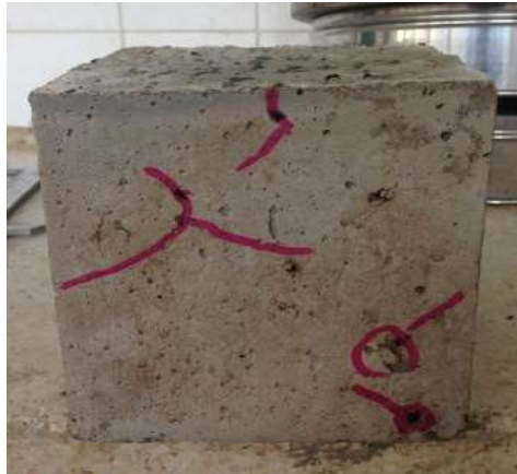
Figure 10: Cube after heating (300oC) in oven for two hours
