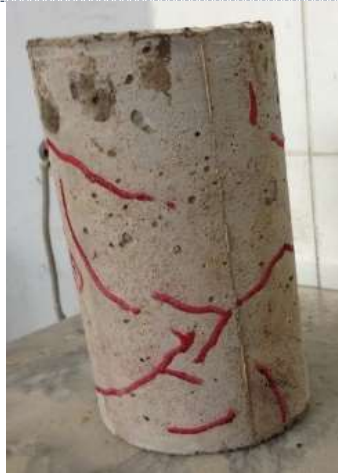
Figure 14: Cylinder after heating (300oC) in oven for two hours
